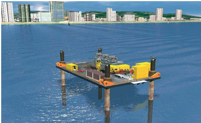
Figure 11.19 A drill rig located at sea on a jack-up platform (Courtesy of Herrenknecht AG)
