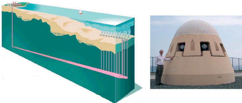
Figure 4.23 Boston outfall schematic and photograph of riser (MWRA)
