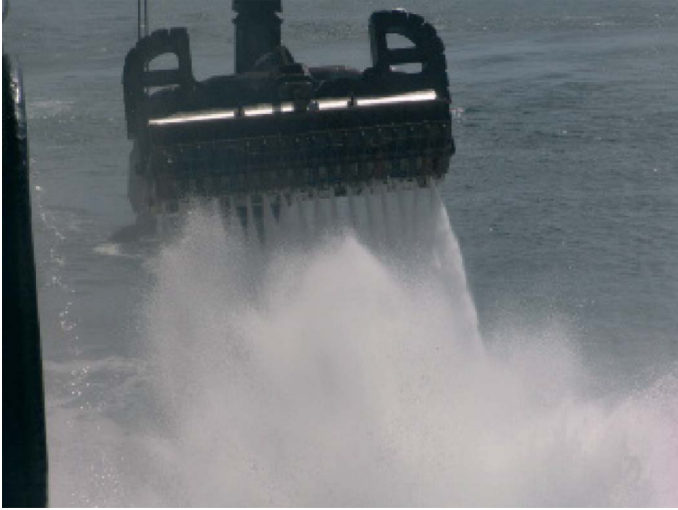
Figure 10.25 Testing the jet nozzle cutter head on a hydraulic suction dredge (courtesy of Bob Dunbar)
