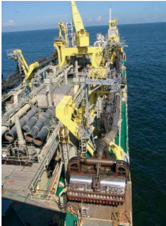
Figure 10.24 Jet nozzle cutter head and suction pipe (courtesy of Bob Dunbar)
