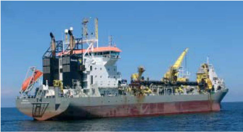
Figure 10.23 A modern jet nozzle suction dredge (courtesy of Bob Dunbar)
