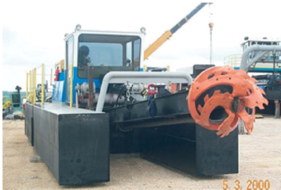
Figure 10.26 Small mechanical cutter head dredge (courtesy of Mud Cat)
