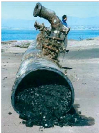
Figure 12.1 Deposits in an outfall diffuser (Pedro Campos, Chile)
