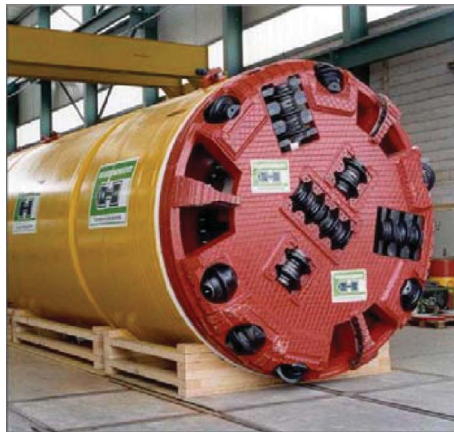
Figure 11.1 Pressure balance TBM with a rock cutting head (Courtesy of Herrenknecht AG)
