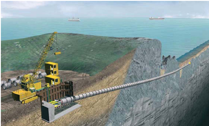
Figure 11.11 Schematic of a jacked outfall from a cliff top (Courtesy of Herrenknecht AG)
