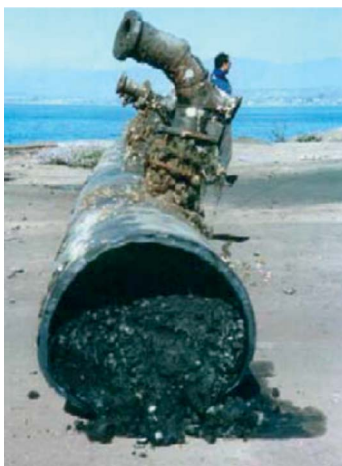
Figure 9.14 Extreme case of diffuser failure due to clogging (Courtesy Pedro Campos)
