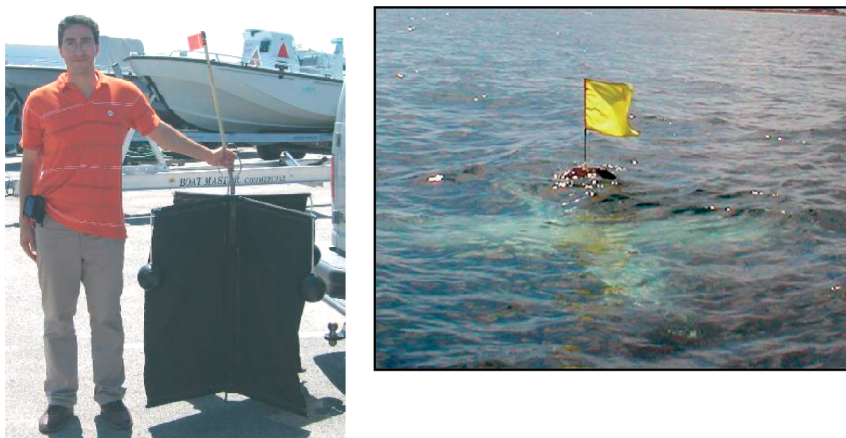
Figure 5.6 Surface drifters (Right, Courtesy Ocean Surveys)
