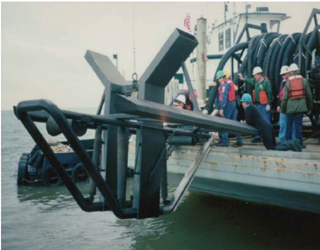
Figure 10.28 Deployment of a small jet sled from the stern of the control barge (courtesy of Bob Dunbar)
